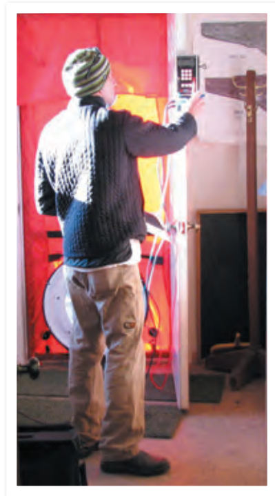
Bill Steyer tests for air leaks
